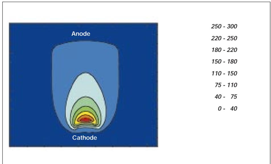
*Fig. 7: Typical luminous intensity distribution in the arc of an HBO® 2001 W/CIL operated at rated power*
