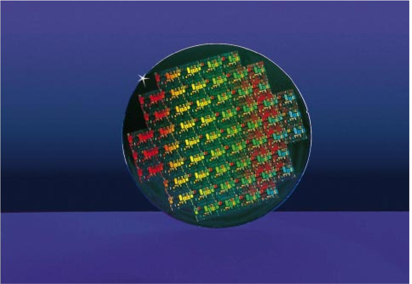
*8-inch wafer with test structure for the development of a 256-Megabit DRAM. This memory chip is based on a 0.25  $\mu\text{m}$  design guideline ("Quarter Micron"). Photo: Siemens AG*
