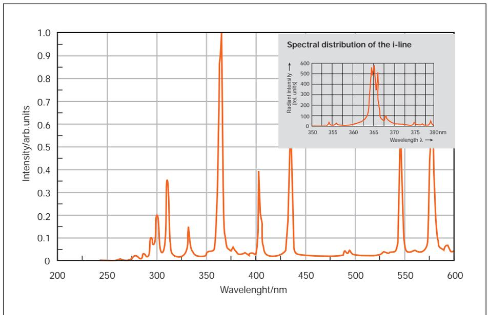
**Fig. 9a: Spectral distribution i-line lamp**
