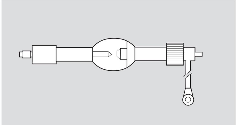
*Fig. 3: Schematic structure of HBO® 1500 W/PIL
