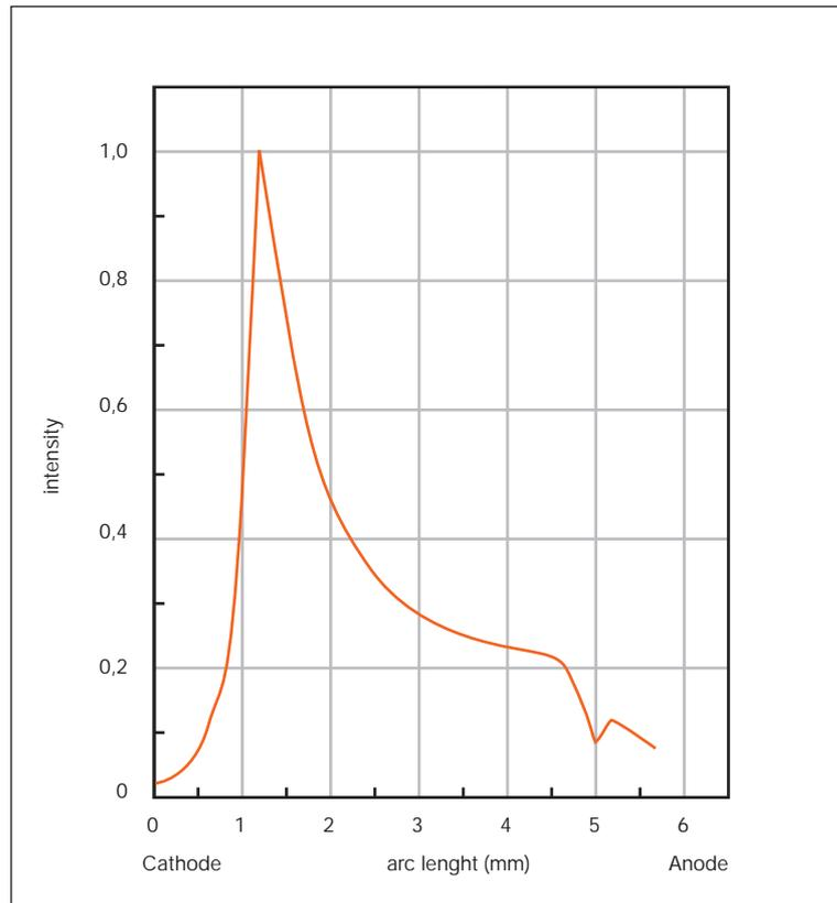
**Fig. 8: Luminous intensity distribution along the arc axis of HBO® 2001 W/CIL operated at rated power**
