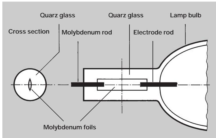
Fig. 4: Schematic diagram of a film seal
