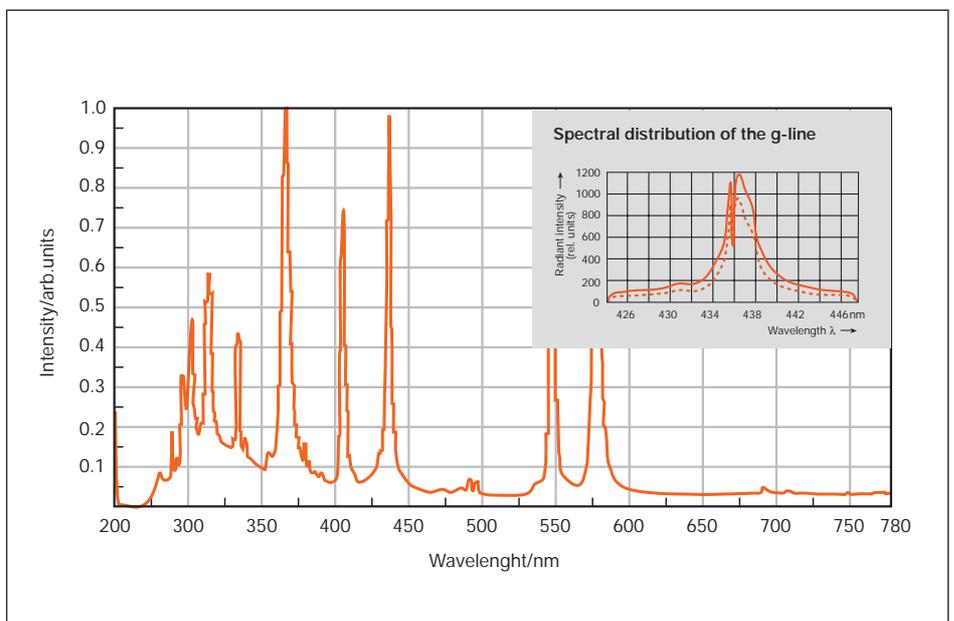
**Fig. 9b: Spectral distribution g-line lamp**
