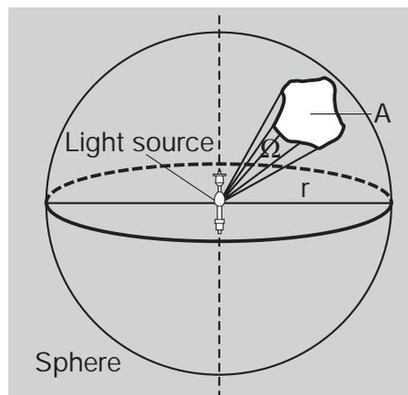
*Fig. 5: On the definition of luminous intensity*
